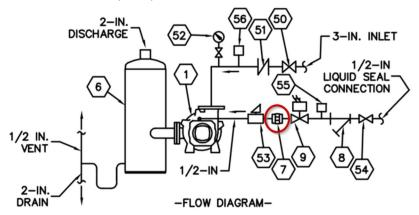
2. Avoid plumbing discharge piping vertically up from the pump. If discharge pipe is vertically above the pump, when the pump stops, the water in the vertical pipe will fall back into the pump, flooding it with excess water. The next time the pump starts, it will try to compress too much water, and it will make a loud screeching noise until it has pushed the excess water out.
