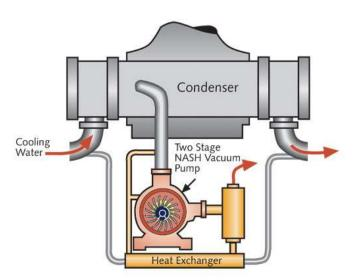
A shell-and-tube, plate-and-frame, or welded heat exchanger can all be an effective condenser solution. However, most processes that need this solution don't produce condensing fluids that are just clean water. Condensable tend to be sludgy and sticky, require regular cleaning of the condensers. Solberg came out with a vapor condensing separator recently, which aims at solving this pain point. See below image.
