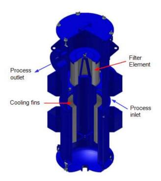
This dual-shelled design allows cooling water to flow through the cooling fins in between the two shells, condenses incoming vapors, which collects at the bottom for periodic discharge and cleaning. A filter element or demister pad can be installed at the top section of this unit to capture fluid droplets and solids. I wish we had one of these units years ago, it would have saved me a lot of pain from brushing out the shell-and-tube heat exchangers we used as condensers.
