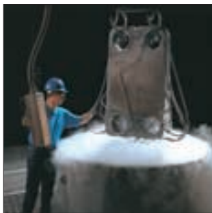
Gasket removal using liquid nitrogen. Complete removal of gasket and glue without damaging the plate.
