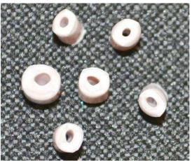
Another damaging effect of not sufficiently removing moisture by vacuum is advanced polymer degradation through hydrolysis. Although plastic products appear to be solid pieces to our naked eyes, on the microscopic level they can be visualized as a mess of entangled and crosslinked spaghetti noodles, or polymer chains. These entangled and crosslinked polymer chains is what gives a plastic product its physical properties: rigidity, ductility, impact resistance, flexibility, etc.
