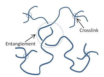
Hydrolysis is the process in which polymers are broken down into monomers when water molecule is introduced. It essentially breaks a long polymer chain to smaller chains, therefore reducing its ability to entangle and crosslink with other polymer chains. Therefore, reducing a plastic product's physical properties, making it more brittle, less flexible, or not withstand against impact.
